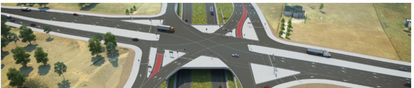
The proposed grade separated interchange (underpass) at The Northern Road and Bringelly Road
