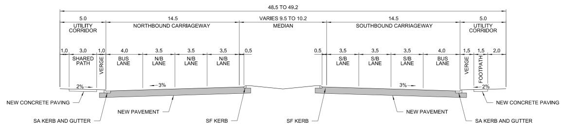
TYPICAL CROSS SECTION - BETWEEN GLENMORE PARKWAY AND M4 MOTORWAY (DIMENSIONS ARE IN METRES)
