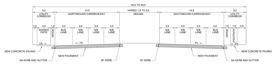
TYPICAL CROSS SECTION - BETWEEN TUKARA ROAD AND MAXWELL STREET (DIMENSIONS ARE IN METRES)
