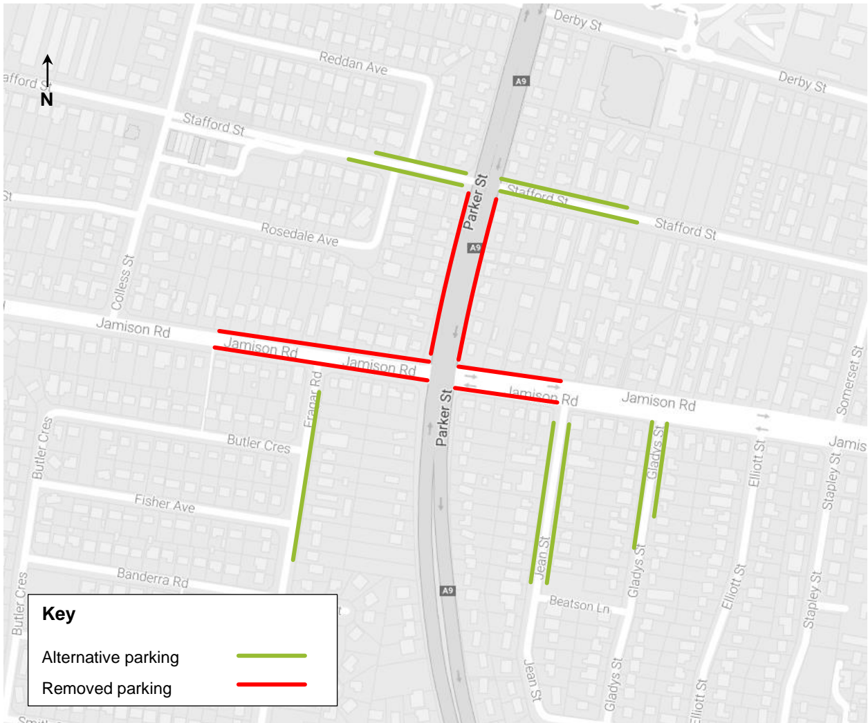
Figure 5.11 : Proposed removal of parking on Jamison Road
