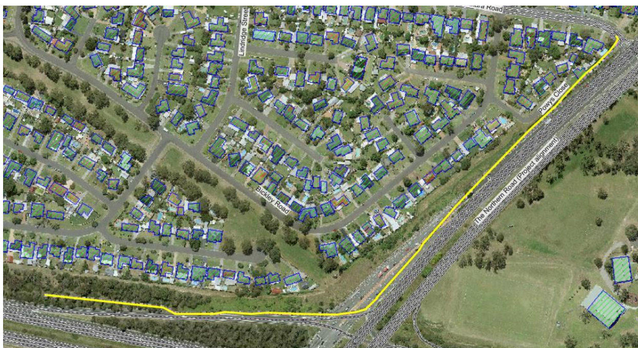
Figure 9-1 Horizontal extent of proposed noise wall at M4 Motorway to Powys Close (noise barrier shown over existing, not future, road alignment)
