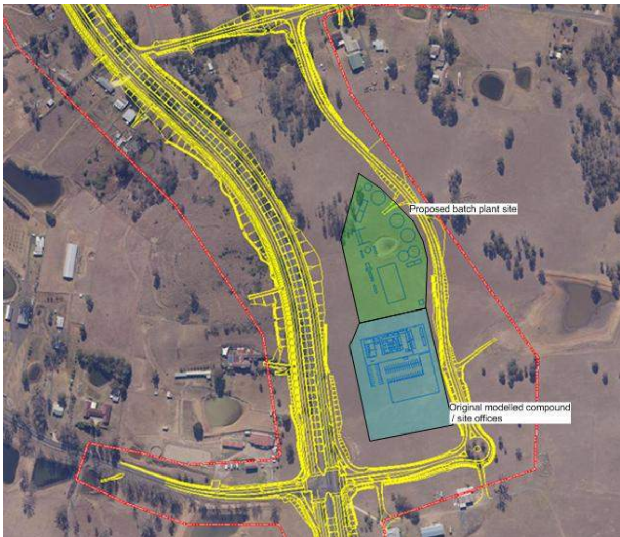
Figure 2.2: Indicative location for concrete batch plant at C16
