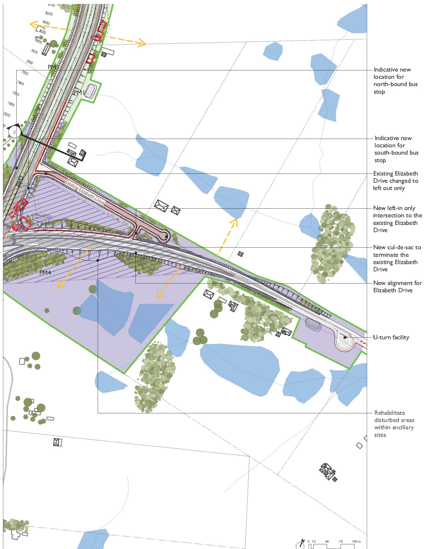
Sheet 8 - Chainage 7,800 to 8,100, including the re-aligned Elizabeth Drive
