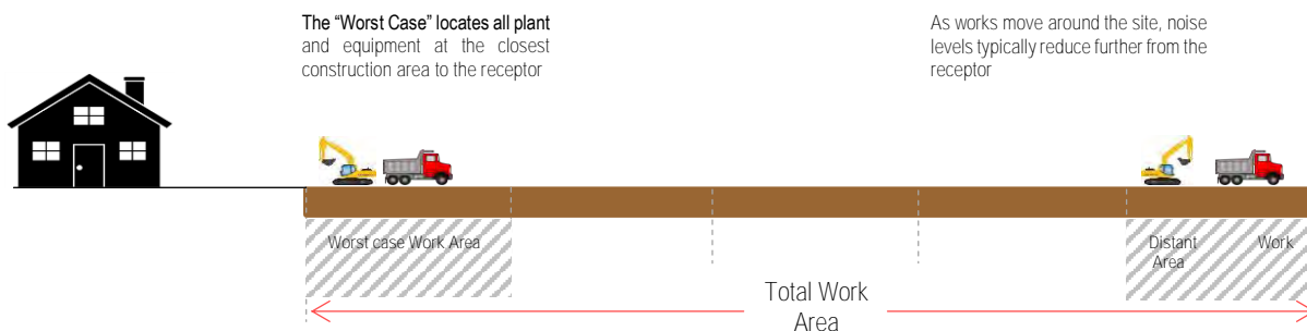
Figure 4 Conceptual Illustration of Work Areas
