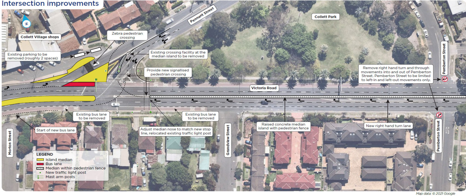
Figure 1: Proposed safety improvements on Victoria Road between Pennant and Pemberton streets, Parramatta
