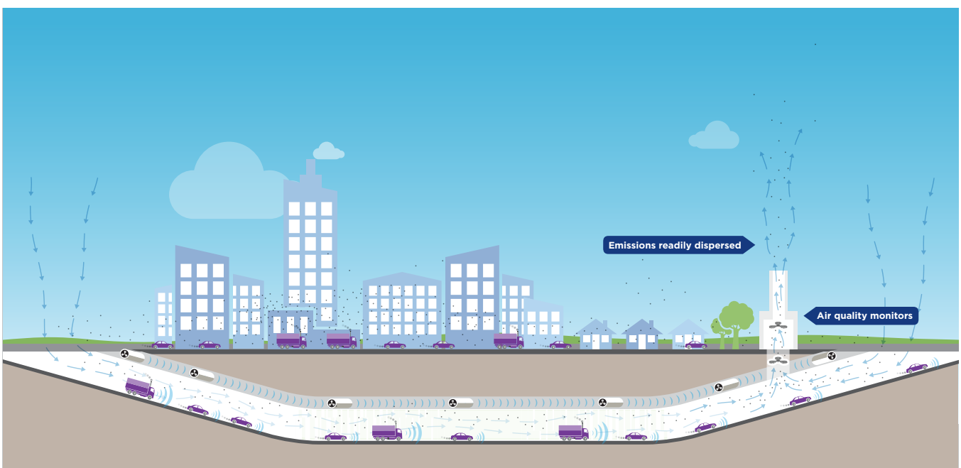
Artist's impression longitudinal tunnel ventilation system
