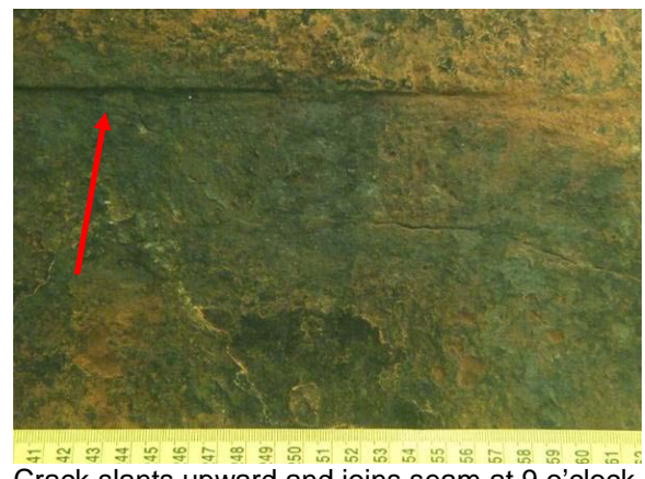
Crack slants upward and joins seam at 9 o'clock (south aspect)
