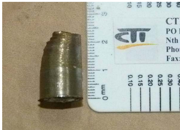
5D NE aspect, above water; no graphitisation
