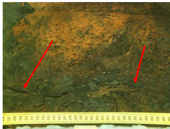
Crack on 6D some 200mm below seam, with occasional frayed edges
