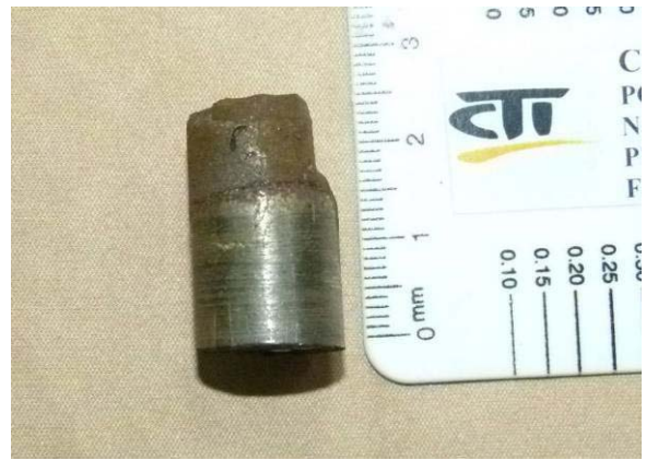
5U NE aspect, upper quarter of immersed casting, showing 9-10mm of graphitisation and 14-15mm remaining cast iron
