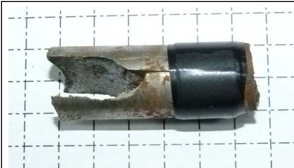
Core from seam between sections as retrieved by divers - length > 50mm, with cast-in rebate for gasket (two halves taped together)
