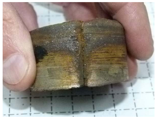
Graphitisation follows line of crack indicating crack to be of reasonable age
