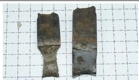
Inner ends of the two halves of the core were a concave shape, indicating the core intersected a bolt hole
