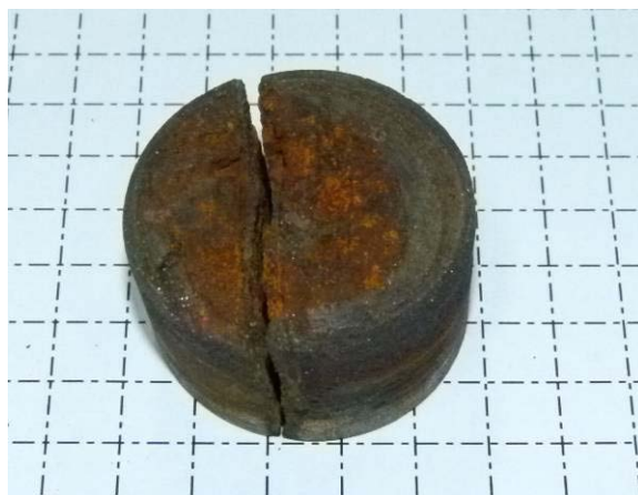
Core (50mm diameter) through crack on 5D showing it to extend full depth through the casting
