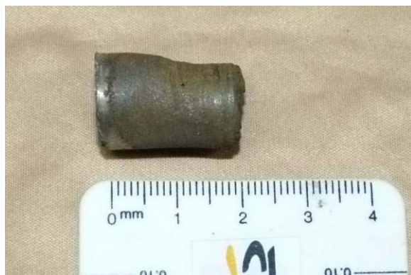
5U SW aspect, upper quarter of immersed casting, showing up to 18 mm of graphitisation and as little as 2mm remaining cast iron
