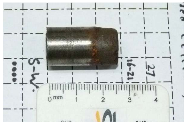
5U SW aspect, lower quarter of immersed casting, showing up to 11 mm of graphitisation and as little as 16mm remaining cast iron
