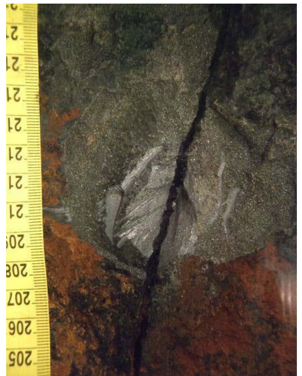
Cleaning and excavating graphite layer shows crack to extend beyond the outer graphite layer
