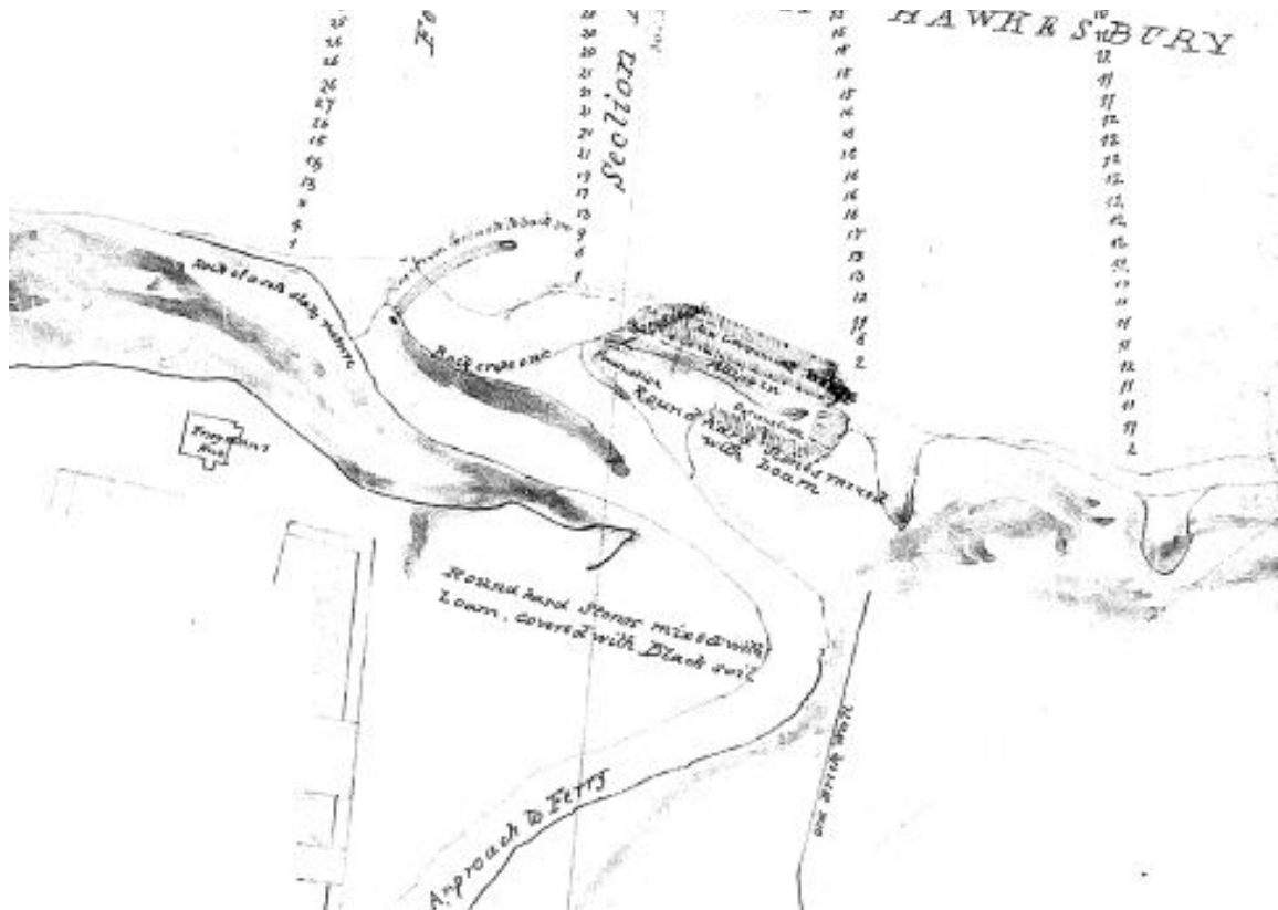
Plate 108: Detail of a survey plan of the proposed bridge location c. 1870. The hand written text on the riverbank identifies the locations of "round hard stones mixed with loam, covered with black soil" in the bend of the road, "Round hard stones mixed with loam" close to the river and it identifies the wharf (shaded area above the curve in the road as "New Government Wharf"). North is up and pivoted slightly to the right. 540
