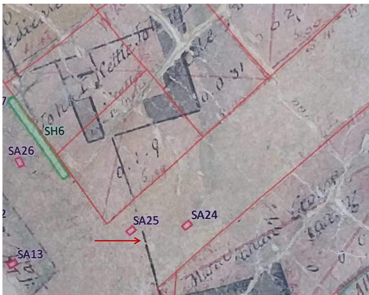
Figure 70: A georeferenced overlay of the location of SA 25 on a map of 1841 showing the Government Domain wall and gateway (red arrow). The wall is very likely to have been rebuilt in brick by this time. (Source: AAJV overlay on 1841 Plan of Windsor, personal reference library of Ian Jack).
