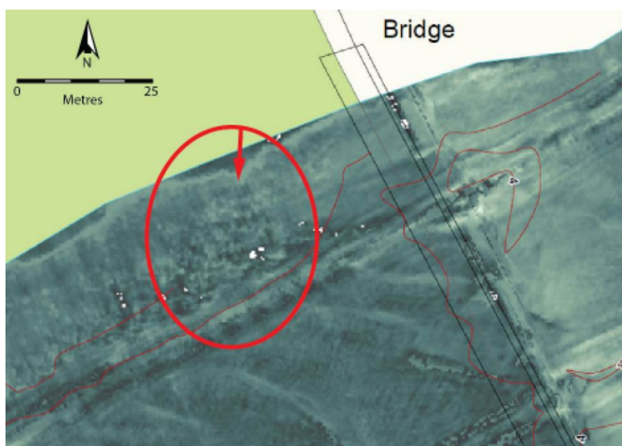
Figure 50: Localised scouring caused by a stormwater drain or similar in this area.
