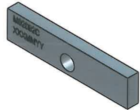
SUPPORT PLATE FOR DETECTOR HOLDER PART NUMBER: M02692C MATERIAL: 40 X 16 FLAT MILD STEEL AS3679-250 FINISH: 1 COAT OF R.O.Z.P.
