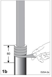
Wrap one layer of long (50mm wide) sealant tape (red) with slight tension starting at the end of the inner sheath downwards for 60mm.
