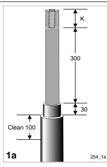
Cables without Insulation Screen Cut the cable to the required length. Remove both the layers of the composite sheath for 300mm + K. K = depth of connector barrel hole + 5mm.
