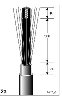
Cables with Insulation Screen Cut the cable to the required length. Remove both the layers of the composite sheath for 300mm + K. K = depth of connector barrel hole + 5mm.
