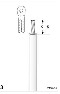
Cut back the insulation according to dimension **K** = depth of cable lug barrel hole + 5mm.
