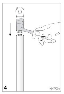
Wrap the short (20mm wide) red sealant tape around the barrel of the cable lug. Stretch the tape to half of its width and apply with half overlap. Use the remaining sealant (red) to fill in the space between the core insulation and the cable lug to leave a smooth transition.
