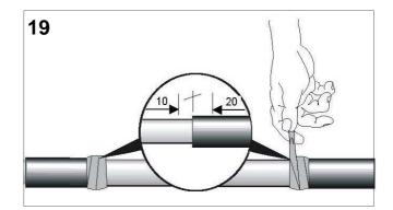
Take the yellow void filling tape from the alu foil packet. Remove one release paper from the strip & roll up. Apply the tape with 50% overlap stretching it to about half its original width.
