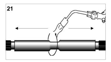
Position the screened insulating sleeves (Y) centrally over the stress control tubing.
