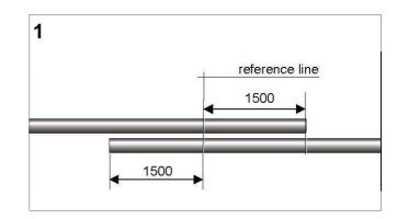
The installation will need 2.5 m of cable on either side of the reference line.
