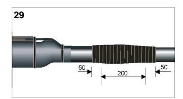
Centre the sealing sleeve (1: WCSM-130/36) over the mastic area. Insert the branch-off clip. Shrink the sleeve into position starting in the centre, working towards the ends.
