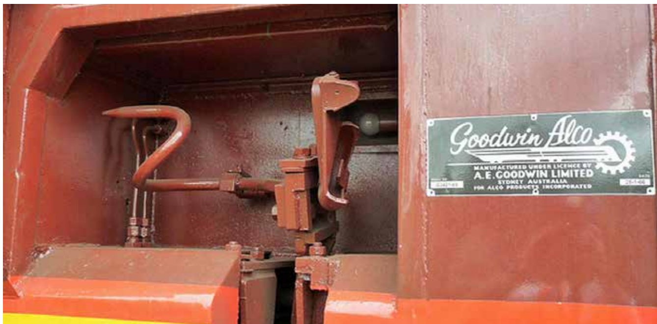
Automatic staff exchange mechanism on train. (NSW Railways Safeworking photo)
