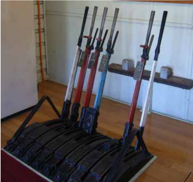
Type-C Standard interlocking machine, Berry Station (Cinétel Productions)
