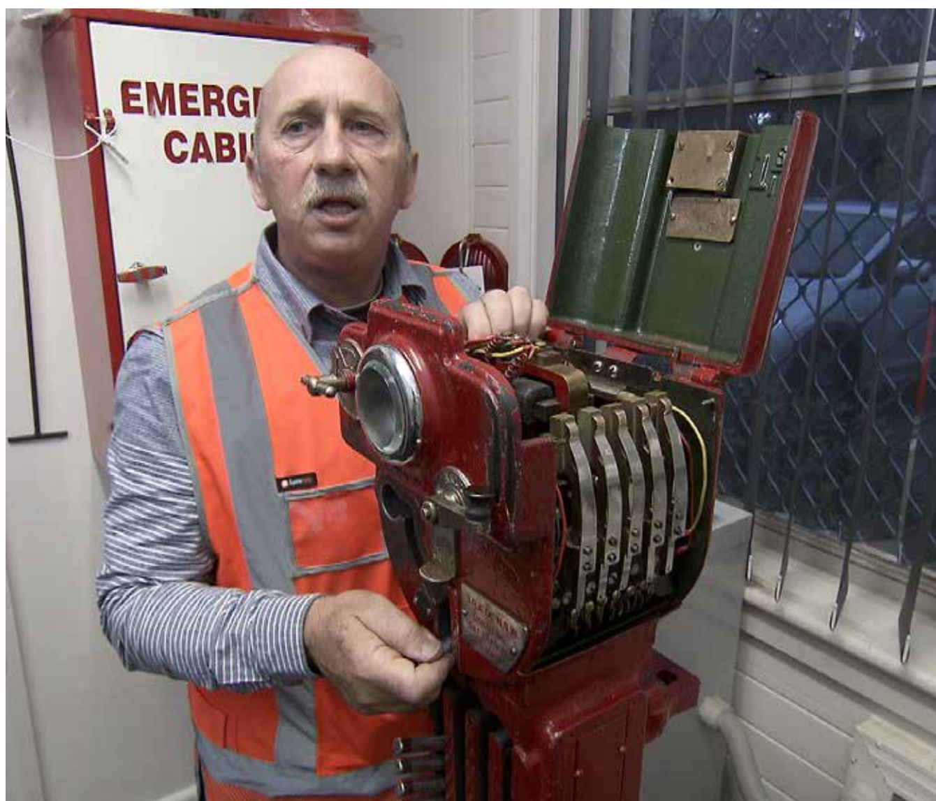
John Rasborsek demonstrating inner workings of ETS instrument. (Cinetel Productions)
