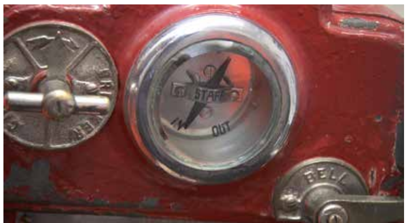
Galvanometer on electric staff instrument. (Cinetel Productions)
