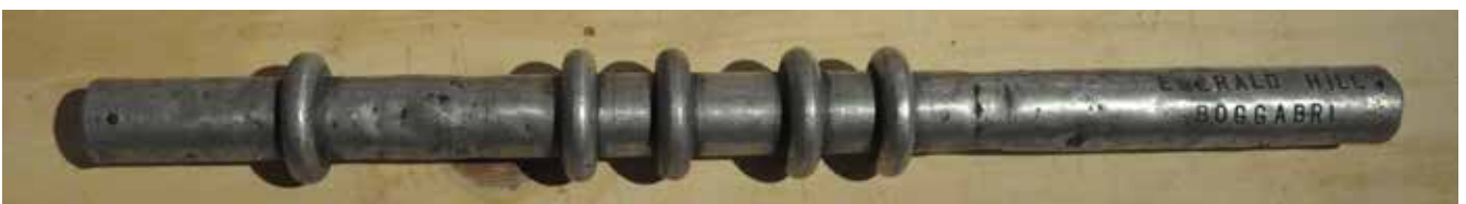
Electric Train Staff, the large and original electric staff system. (Courtesy Robert Taaffe)
