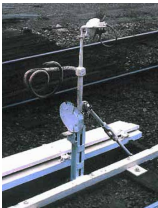
Automatic staff exchange apparatus, Culcairn 1980s. (NSW Railways Safeworking photo)
