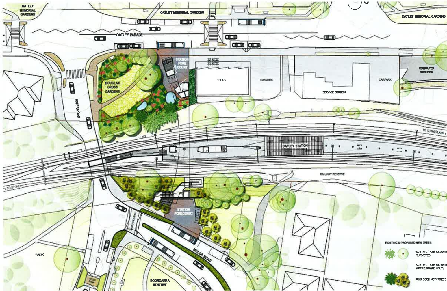
Figure 29: Site plan for developed option 2 (the proposal), with a curved footbridge and reduced forecourts.
