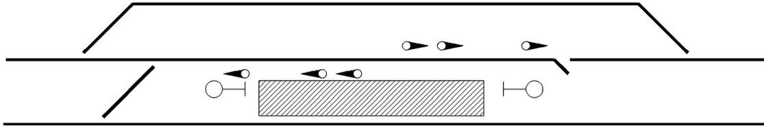
These ITS are provided to prevent catchpoint runoff in tight situations. Short (4 and 6 car) trains are prevented from achieving any run up by the additional ITS located just past the 4 and 6 car mark. If these trainstops are suppressed for departing trains, this protection is removed just at the time it is most likely to be required, should the train move the wrong way.
