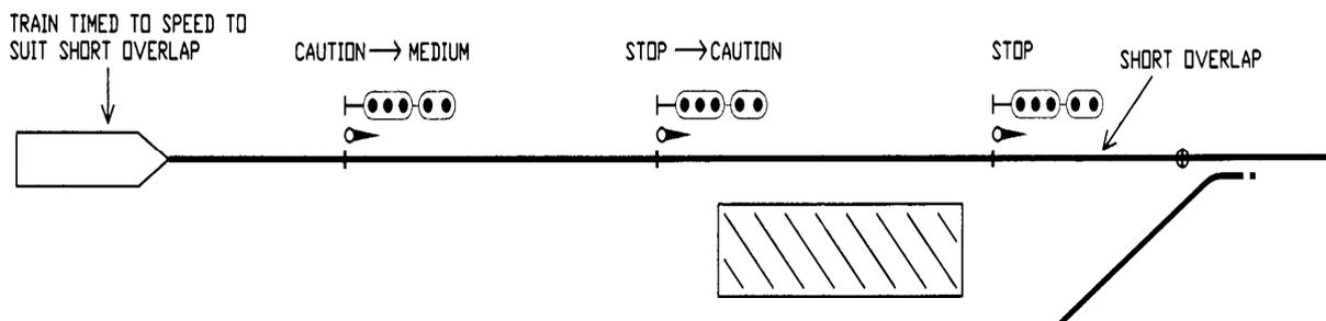
For this to be effective, the train must be well in advance of the conditional medium signal so that the driver may observe the indication.
