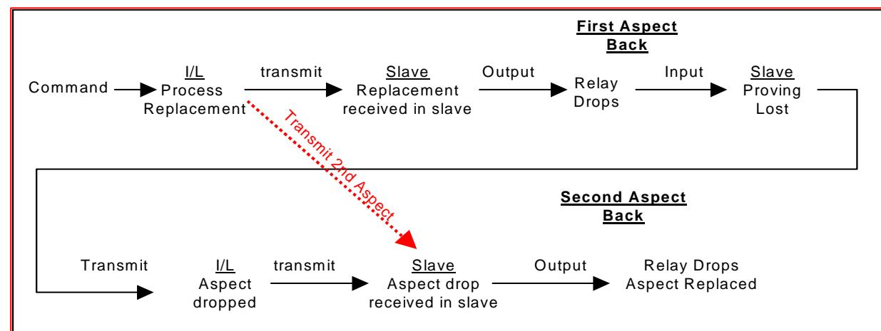
This diagram shows that the two aspects will now restore simultaneously.
