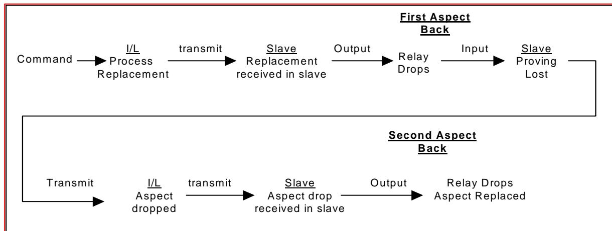
During this period an irregular aspect sequence may be observed if all signals were able to be seen together. However, the situation is safe as in the scenario of an aspect replacement, approach locking would hold the interlocking and is designed to specifically cover this situation.
