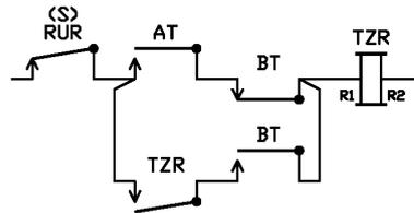
When the shunt route is set, the RUR picks and the TZR drops out. While the B track remains occupied, the TZR will not pick again, and in this case the ALSR must either time out or the approach path must be clear for the route to normalise.
