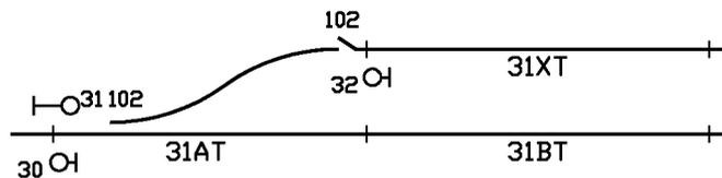
Where the A track has facing points, the B track will be different depending on the lie of the points. The correct B track must be selected to ensure that approach locking cannot be compromised by a train on the "wrong" B track, but can still be released by the passage of the train. Similar selection is required in Options 1 and 2.
