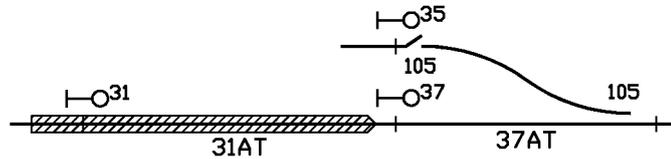
In limited circumstances, where required for operating purposes, an existing route release timer can be used to qualify the A track in the approach lock release.
