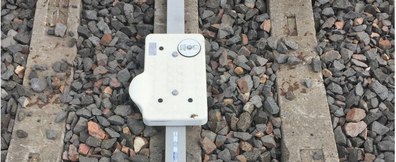
Picture of a 'balise' – an electronic transponder that monitors train speeds.
