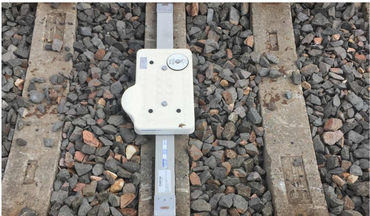
Picture of a balise, an electronic transponder that monitors train speeds.
