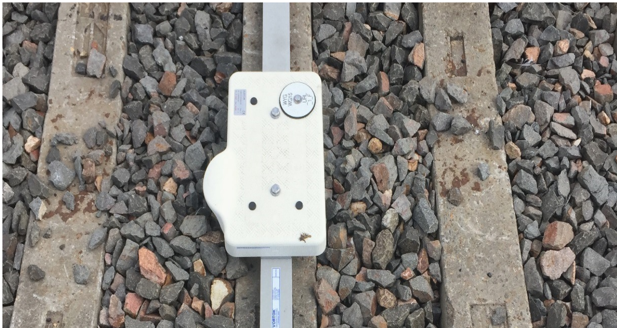
Picture of 'balise' – an electronic transponder that monitors train speeds
