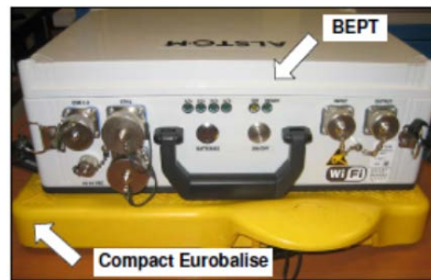
Figure 13 BEPT placement for balise programming
