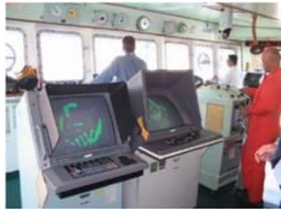
Bridge showing pilot scanning ahead and radar screens and instruments (above the pilot's head) which may need to be read. The master and helm, who are integral to Bridge Resource Management, are also shown.
