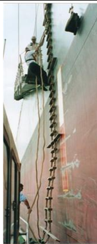
Pilot on ladder using man-ropes reaching accommodation ladder. Cutter below with crew man holding man-rope.
