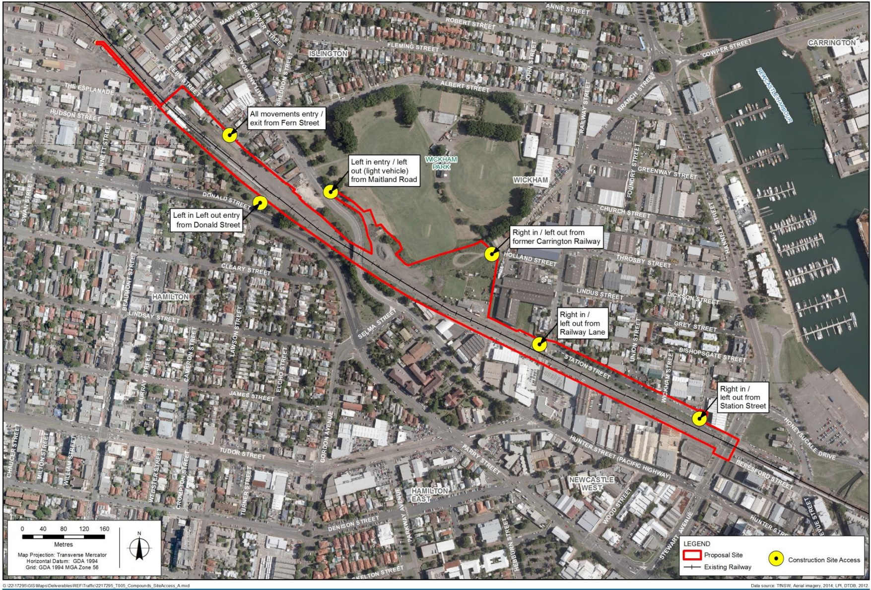
Figure 3.4 Site access points and construction compound
