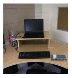
Set Screen Height so top edge of screen is at eye level. This corrects neck posture to minimise loading
