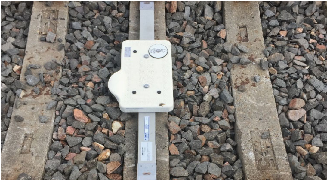
Picture of a balise, an electronic transponder that monitors train speeds.
