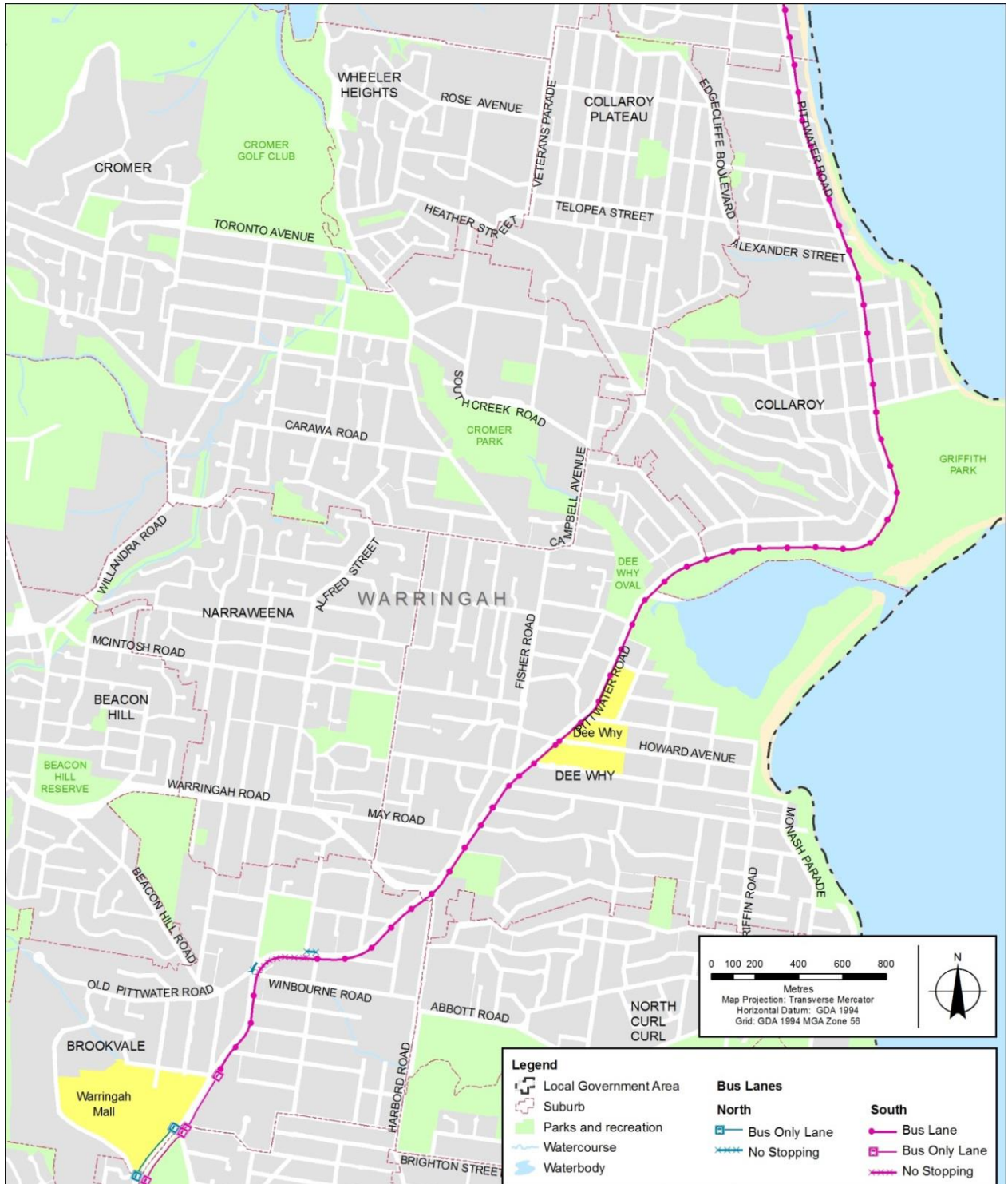
Figure 15 AM peak bus lanes and T3 lanes in Brookvale and Dee Why
