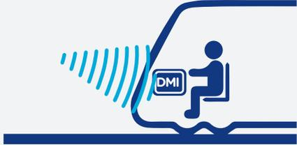
**Replacing traditional trackside signalling equipment** with the latest 'in cab' train control technology (European Train Control System Level 2).
