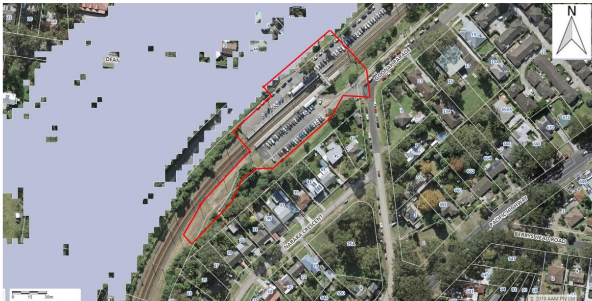
Figure 6-17 Extract from the CCC online maps (CCC, 2020) depicting modelled 1 per cent AEP flood event (shaded grey) with respect to the Proposal area (indicated by the red polygon)
