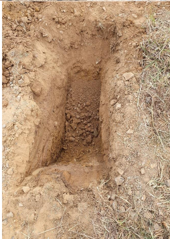
Figure 2.1.5 to 2.1.11 – Test pit location, samples and soil profile.
