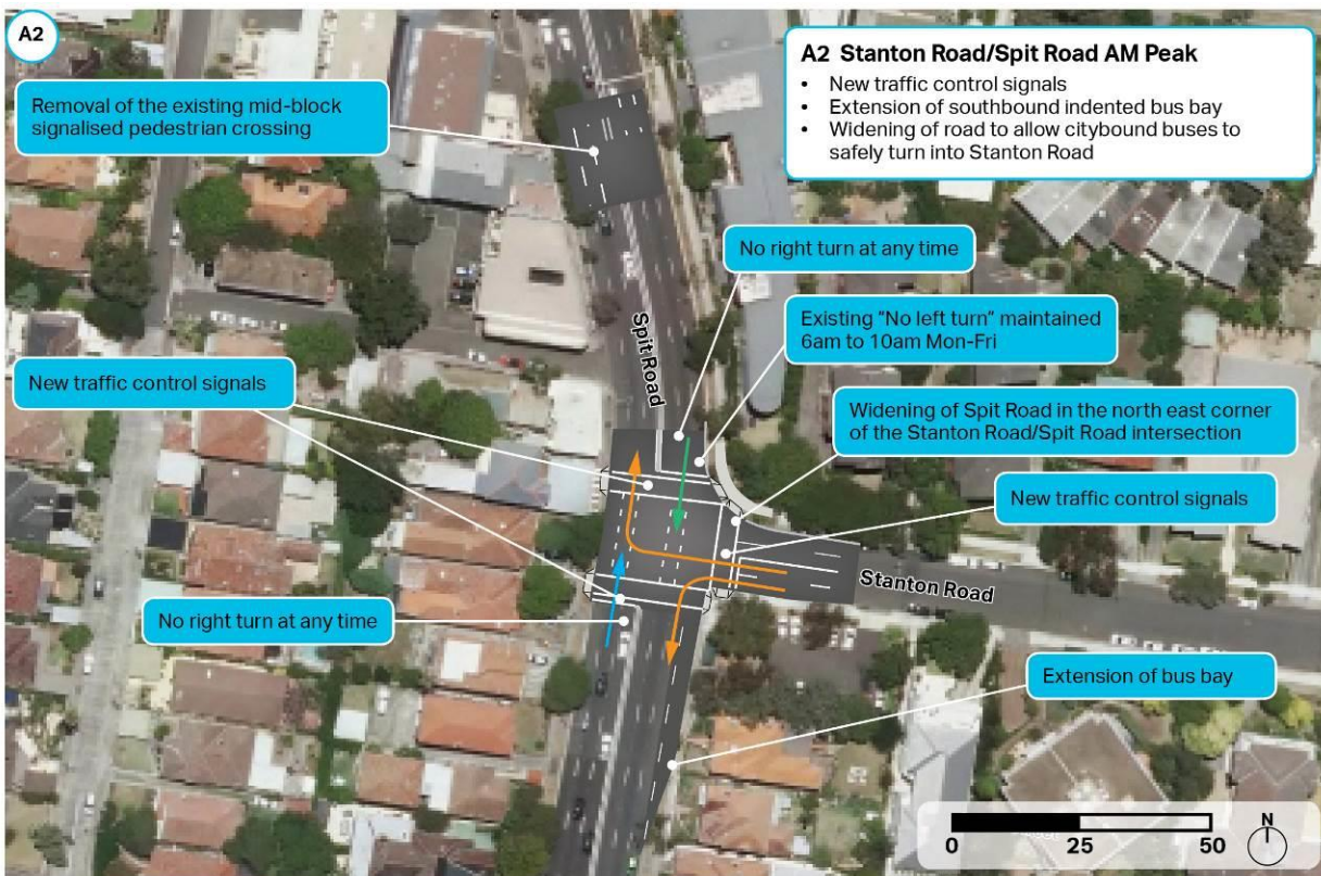
Figure 2-2: Allowable traffic movements at the intersection of Spit Road and Stanton Road during the AM peak.
