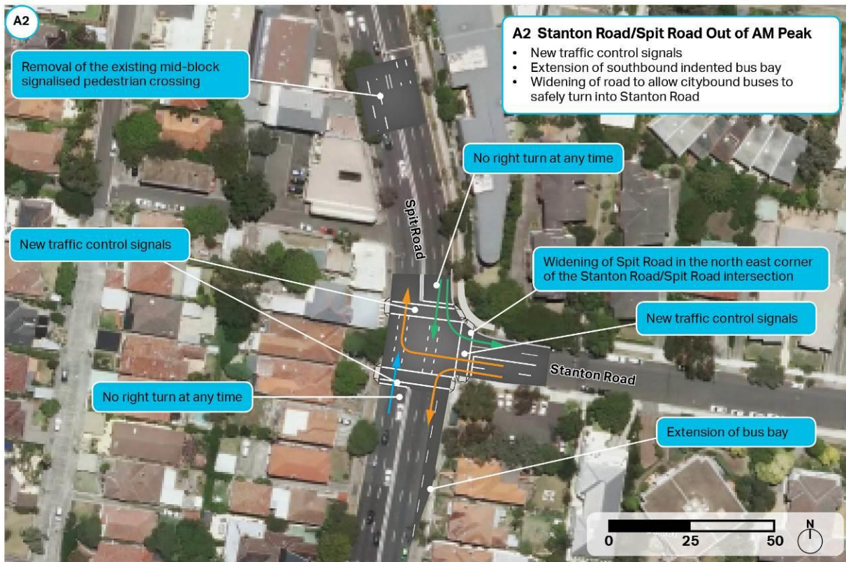
Figure 2-1: Allowable traffic movements at the intersection of Spit Road and Stanton Road outside of the AM peak.
