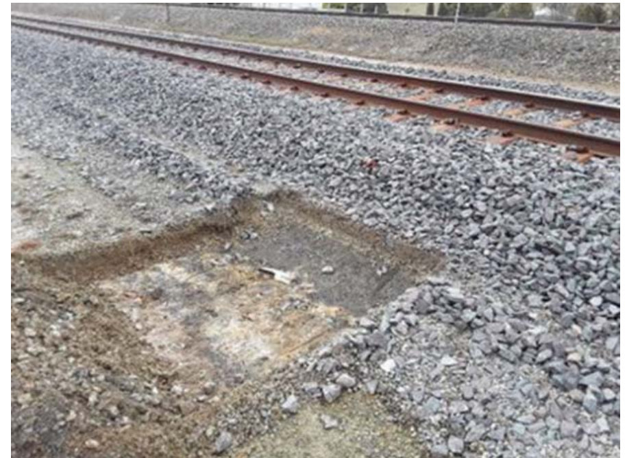
Shallow test pit at northern portion of rail formation
