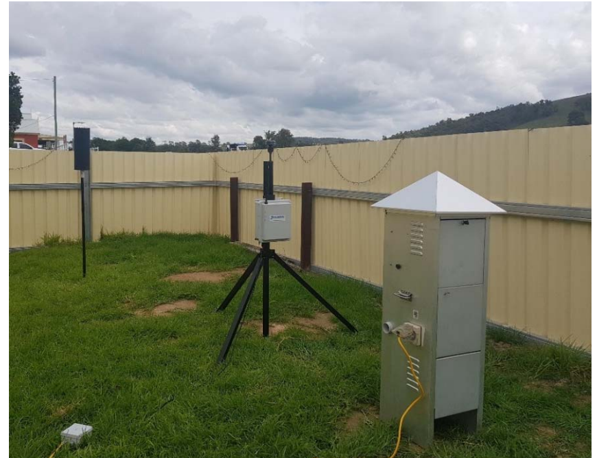
Air quality monitoring station at Goulburn Street
