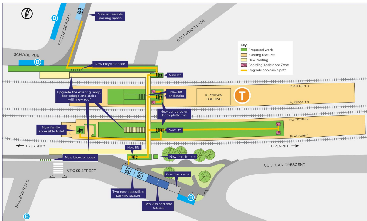
Figure ES.1-1 Key features of the proposed Doonside Station Upgrade (subject to change during detailed design)
