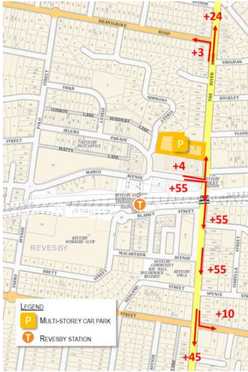
Figure 9 Additional trips generated by the proposed Revesby MSCP extension (PM peak hour)
