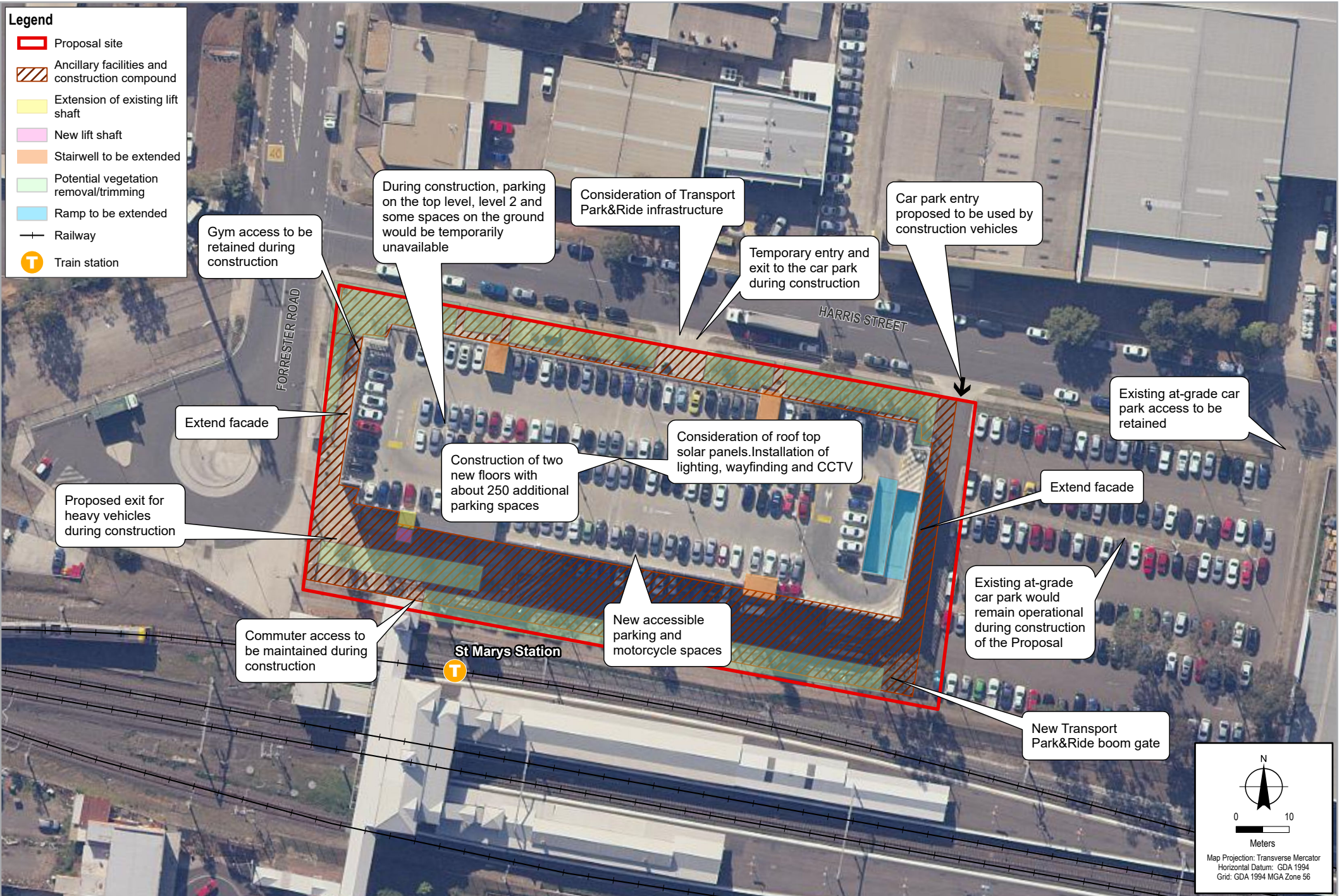
Figure 2 Key features of the Proposed Activity (indicative only, subject to detailed design)
