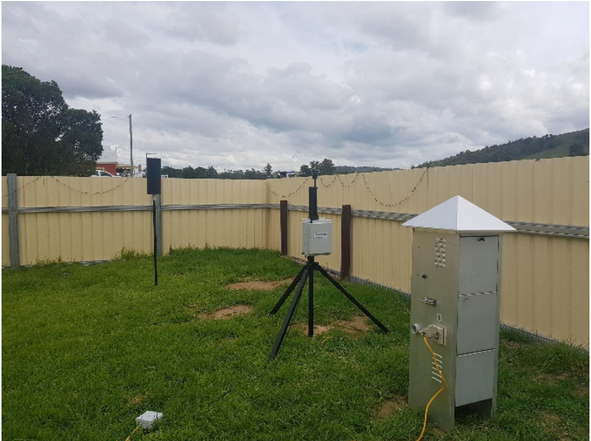
Figure B: Dust deposition gauge (DDG2), particle counter and high-volume air sampler at Station Masters Cottage, 106 Goulburn St, Tarago NSW
