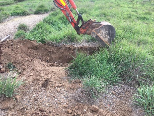
Photo 13 In the uncapped areas the soil profile generally comprised a brown silty sand topsoil with minor fill (to a maximum depth of 0.6 mbgs) with underlying natural clay. Date:01/04/20
