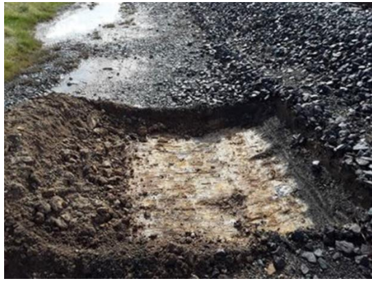
Photograph 37: Composite sample RRE_TP01 collected from shallow test pit adjacent the northern portion of the rail formation. Sample collected 19 August 2020.
