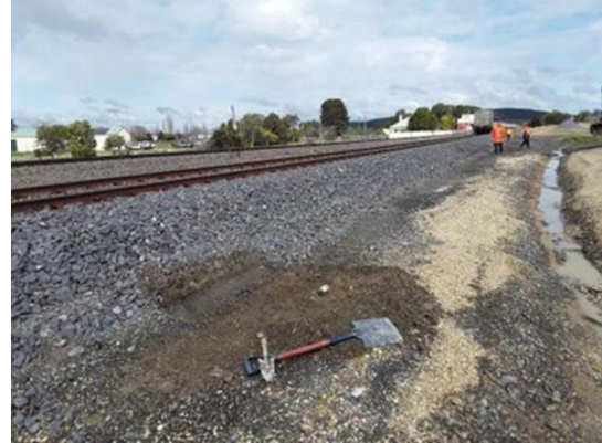
Photograph 40: Composite sample RRE_TP04 collected from shallow soil adjacent the rail formation. Sample collected 19 August 2020.
