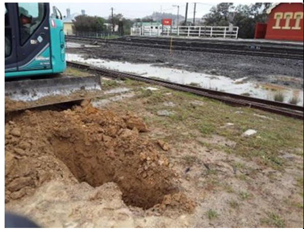
Photograph 28: Test pit LO_TP02 located within the footprint of the former Loadout Facility. Sampled 19 August 2020.
