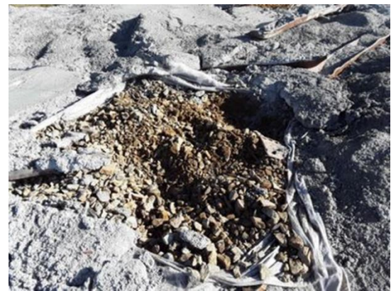
Photograph 52: Composite sample RRE_SP06 collected from the eastern face of onsite stockpile comprising fouled ballast impacted by ore concentrate. Sample collected 19 August 2020.
