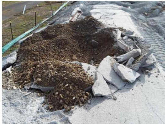
Photograph 55: Composite sample RRE_SP09 collected from the western face of onsite stockpile comprising fouled ballast impacted by ore concentrate. Sample collected 19 August 2020.
