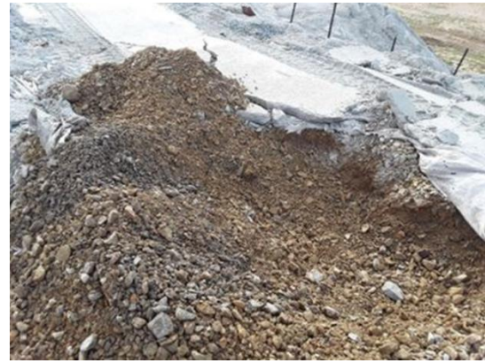
Photograph 56: Composite sample RRE_SP10 collected from the western face of onsite stockpile comprising fouled ballast impacted by ore concentrate. Sample collected 19 August 2020.
