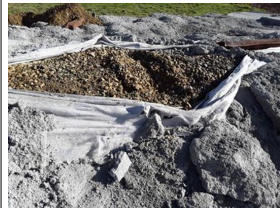
Photograph 51: Composite sample RRE_SP05 collected from the eastern face of onsite stockpile comprising fouled ballast impacted by ore concentrate. Sample collected 19 August 2020.
