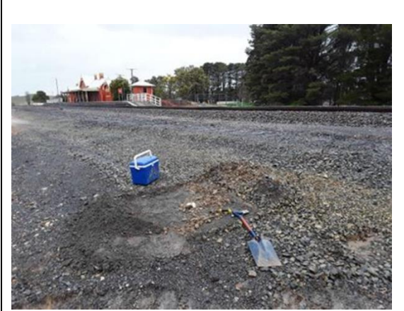
Photograph 45: Composite sample RRE_TP09 collected from shallow test pit adjacent the southern portion of the rail formation. Sample collected 19 August 2020.
