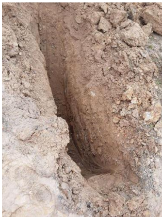
Photograph 29: Test pit LO_TP02 terminated at 1.5 mbgl.
