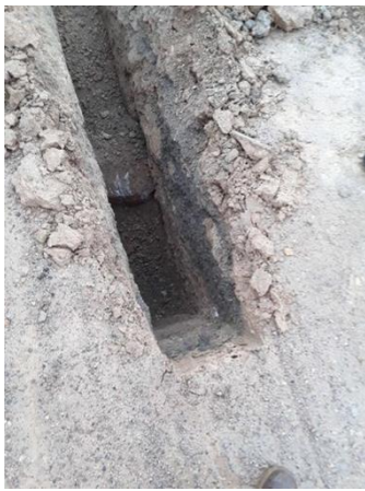
Photograph 27: Test pit LO_TP01 terminated at 1.3 mbgl, refusal on boulder.
