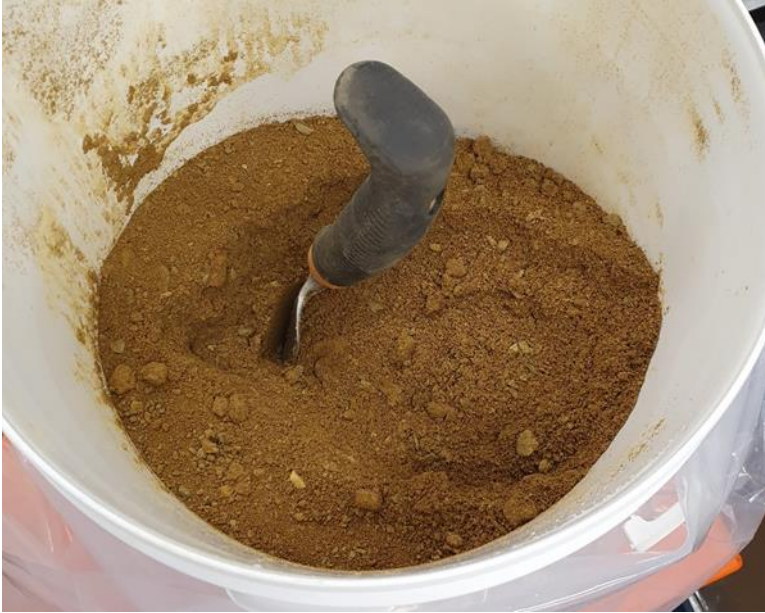
Figure 3. Homogenised bulk sample TP3A used in the lead immobilisation trials.
