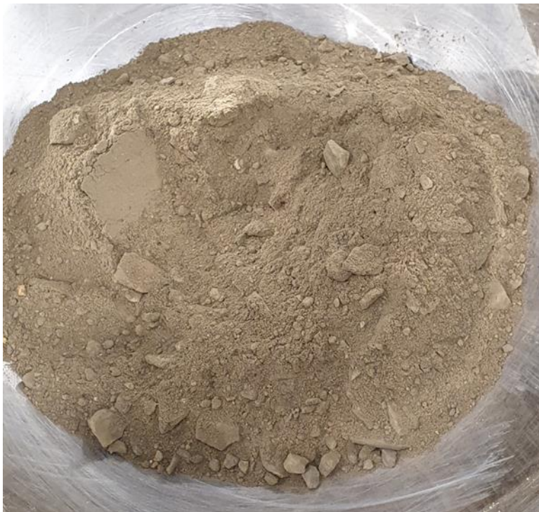
Figure 4. Homogenised bulk sample TP5A used in the lead immobilisation trials.
