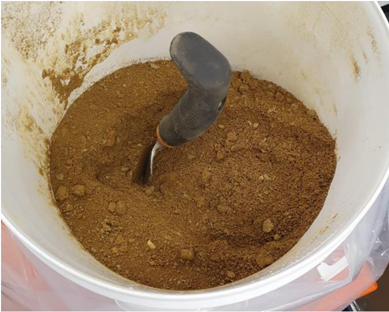
Figure 4. Homogenised bulk sample TP5A used in the lead immobilisation trials.
