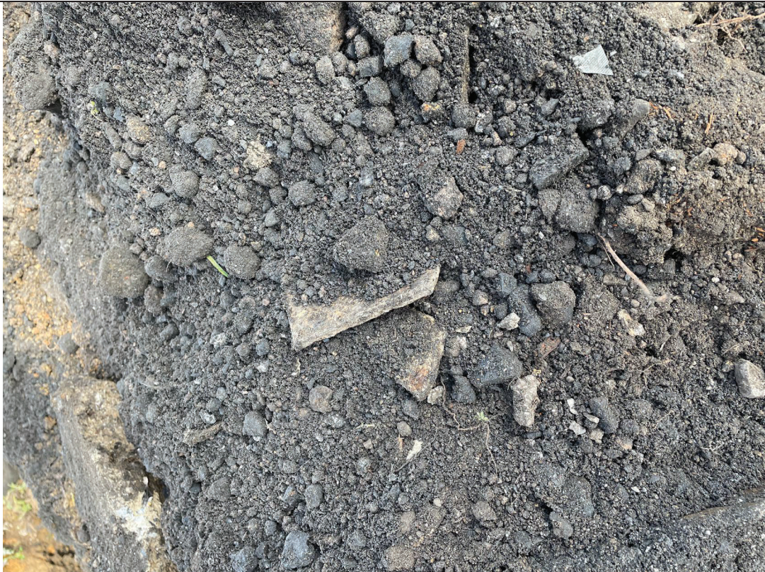
Photograph 17 Asbestos fragments observed within fill material from 1.7 metres in depth during the advancement of TP30.
