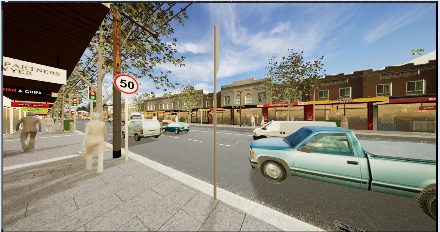
Figure 26: Screenshot of perspective view in game engine immersive virtual environment showing the four lanes with 'Signalised crossing short-wait' (pedestrian prioritised) scenario.
