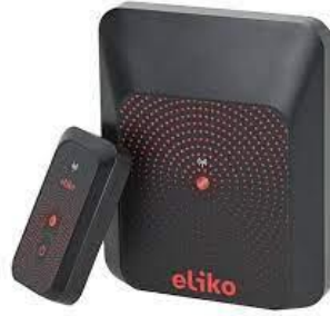
Figure 8. Eliko UWB Locator Tags
