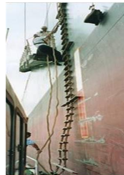
Image 19. Pilot on ladder using manropes reaching accommodation ladder. Cutter below with crew man holding manrope.
