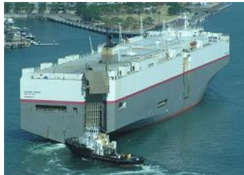
Image 5. Tug manoeuvring the ship under radio-control from pilot
