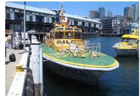
Image 14. Pilot cutter showing handrails, open non-slip surface and marked area for ladder work.
