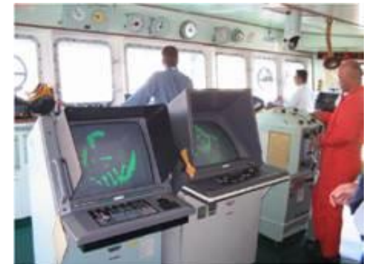
Image 8. Bridge showing pilot scanning ahead and radar screens and instruments (above the pilot's head) which may need to be read. The master and helm, who are integral to Bridge Resource Management, are also shown.
