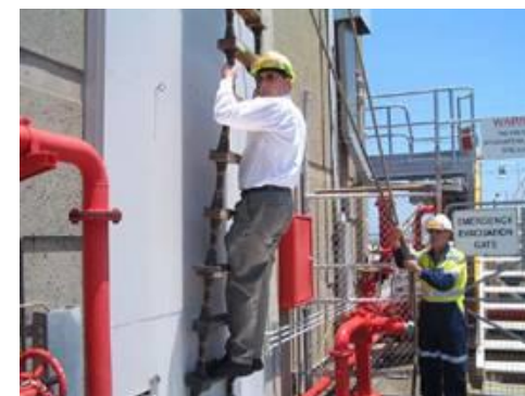
Image 18. Pilot ladder showing use of side-ropes on ladder (on land). (The manropes are being held to one side for illustration purposes.)
