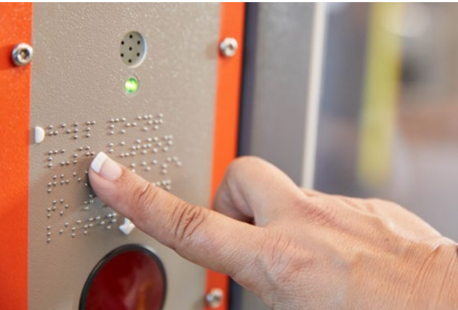
Mariyung fleet - accessible help points with Braille and tactile instructions located next to every allocated wheelchair seating space and in every entry vestibule.
