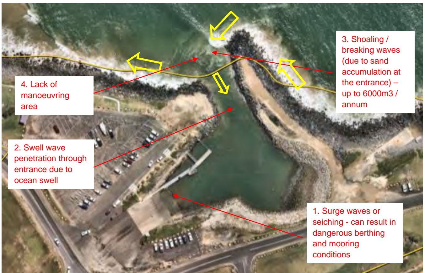
Figure 15: Key Coastal Processes affecting Boating Safety at the Coffs Harbour Boat Ramp facility
