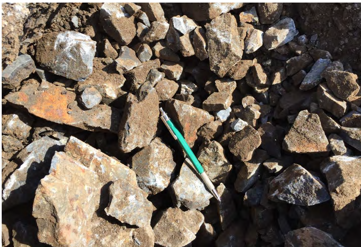
Photo 7: Image of Bridging Rock Beneath the Boat Ramp Car Park
