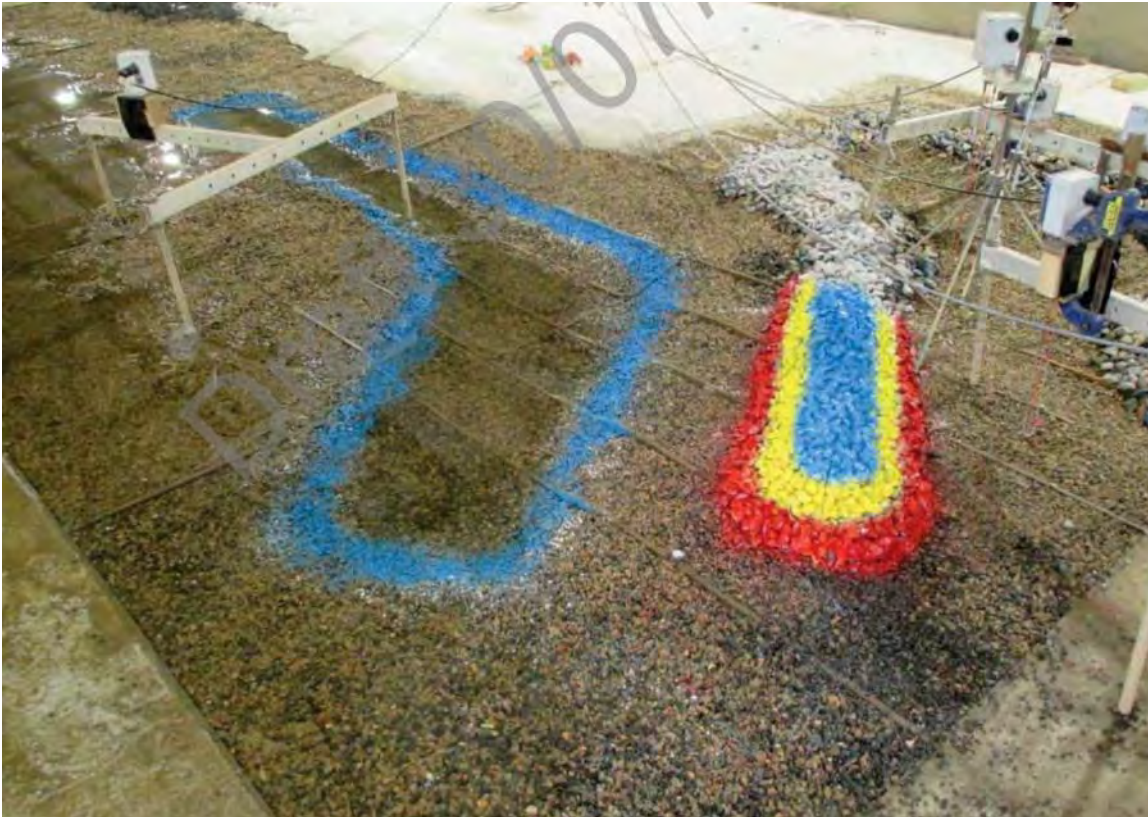
Figure 17: Physical Model at Manly Hydraulics Laboratory of Proposed Coffs Harbour Boat Ramp Breakwater Extension and Offshore Dredged Sediment Sink Concept (MHL, 2020)
