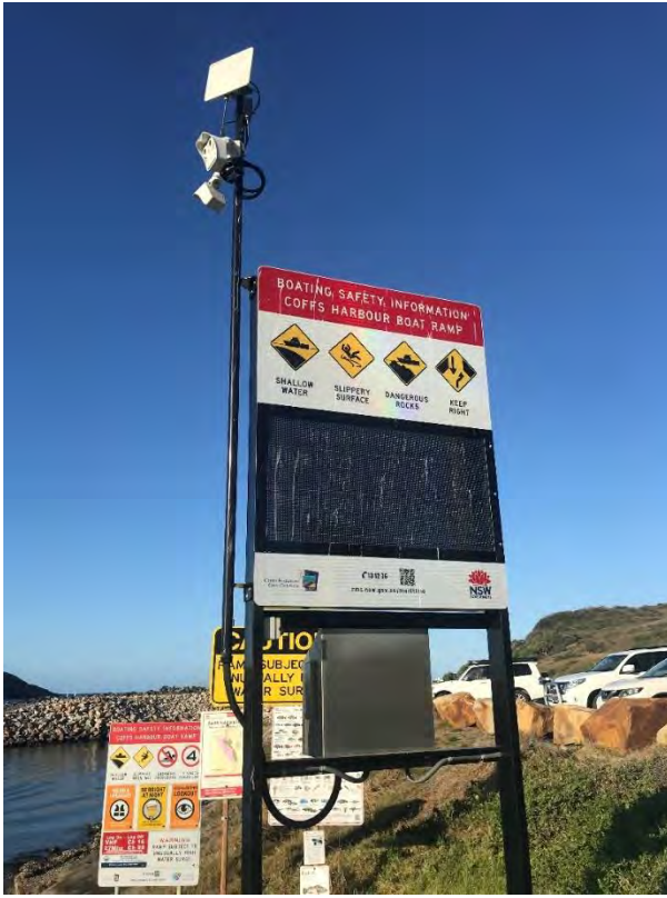
Figure 13: Photo of the automated RMS Boating Safety Information Sign
