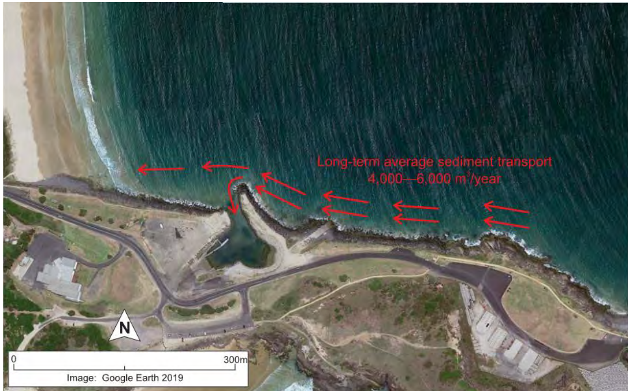
Figure 6: Existing sediment transport pathway along southern shoreline of Coffs Harbour (Source: MHL 2019)
